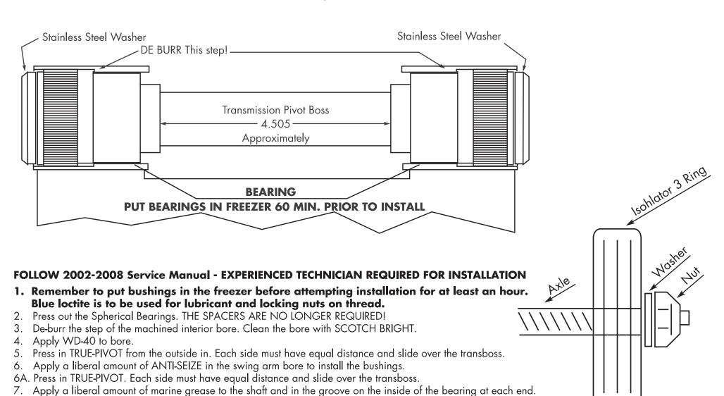
9. Do not tighten nuts to spec until the bike is sitting on the ground at ride height.
