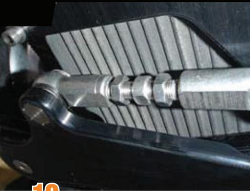
**10** The heim joint is pre-set from True-Track; however, each frame is different and thus some adjustment may be needed, which is why left- and right-hand threads are provided. It is critical that the heim joint be neutral before locking down the jam nuts.
