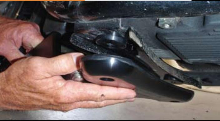
**6** We then lifted the True-track assembly into position and with some thread locker on the bucket bolts that were included, we loosely threaded the bolts into the trans pan and then aligned the dog bone with the cross member and pucks.
