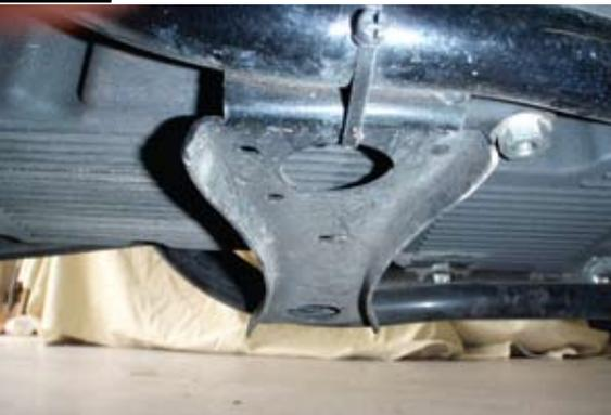
**5** The bucket will mount to the back of the transmission. So we removed the five stock mounting bolts from the back of the transmission pan.
