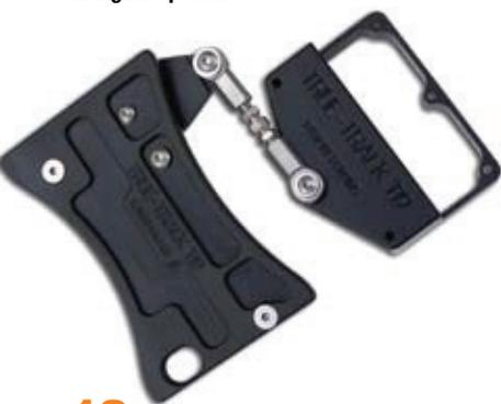
**12** Here is what the True-Track unit for the new '09-present touring models looks like. Installation is essentially the same except it takes a little bit longer on bikes with the crossover pipe running under the bike, as the left-side saddlebag and exhaust have to be removed and reinstalled. Notice the dog bone on this unit is much larger.
