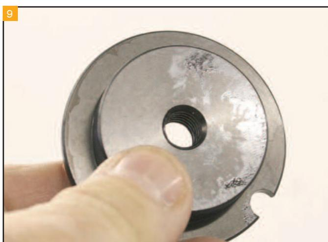
This is one of two discs that will hold the dogbone integration device in place.
