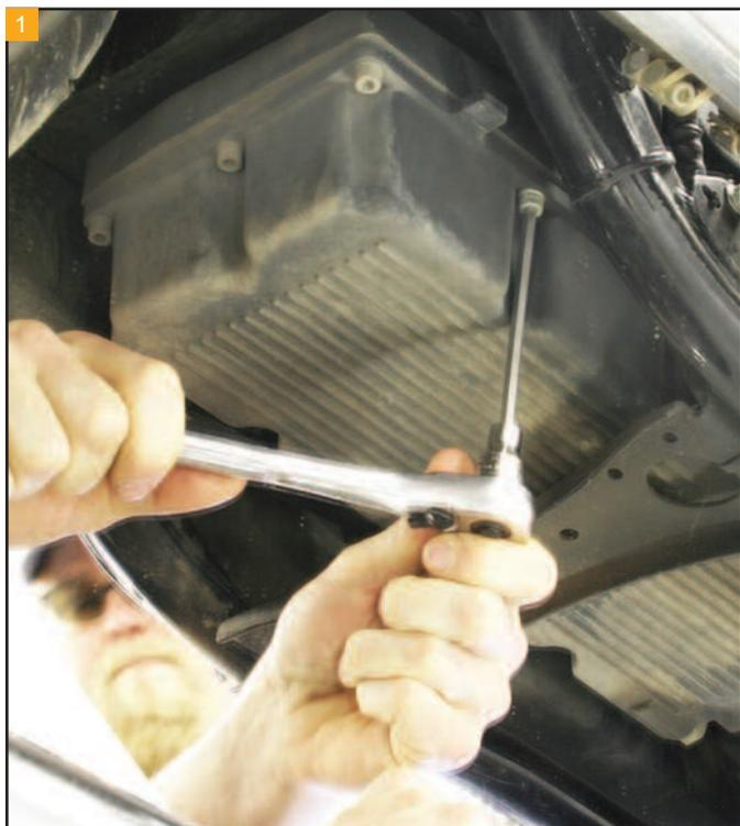
1 Loosen and remove the bolts holding the oil pan in place.
