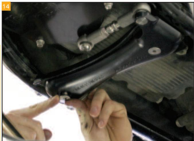
Fit the link in place and install the hardware. Install the dogbone hardware to hold it in place.
