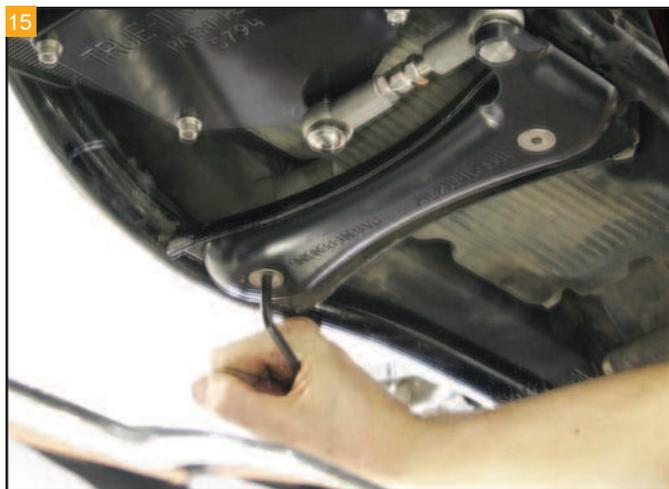
Tighten the dogbone hardware equally on both sides.
