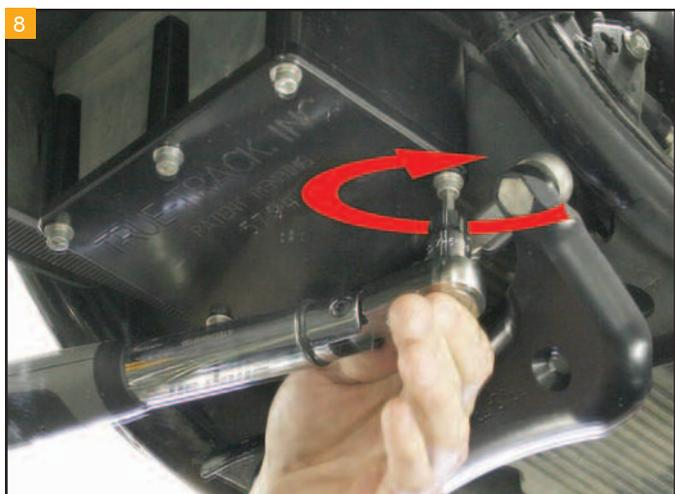
Using a quality torque wrench, torque the pan bolts only after complete assembly.
