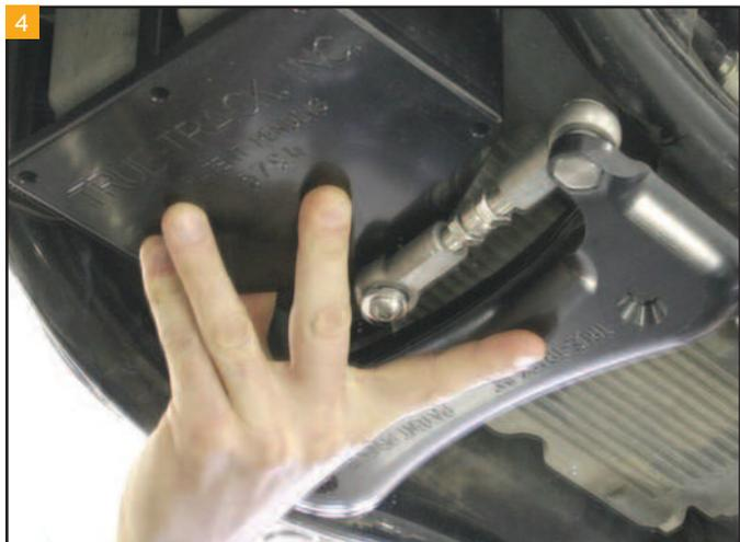
Fit the True-Track into place. True-Track brackets are assembled from the factory – **Do Not Disassemble**.
