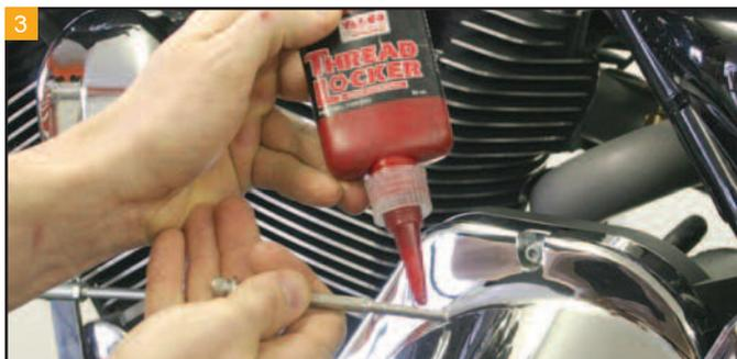
3 We're using Theadlocker on all the True-Track hardware for a secure lock. True-Track advises Blue Loctite on all hardware threads.
