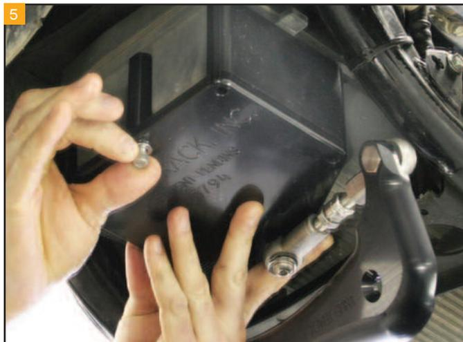
Then, install the True-Track hardware to hold it in place.
