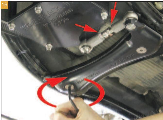
16 Make sure that the link isn't in a bind as you tighten the dogbone hardware.
